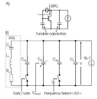
Figure 3: A) VCXO simplified circuit, B) VCXO model.
