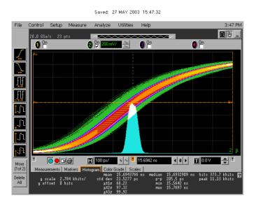
Figure 4 Long term jitter histogram for the QPLL driven by the TTCrx with high density data.
