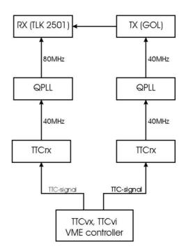
Figure 5 : BER test set-up
