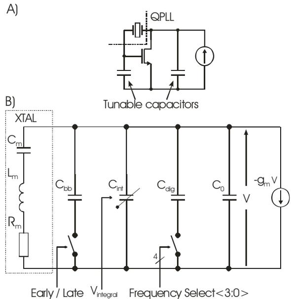
Figure 3: A) VCXO simplified circuit, B) VCXO model.
