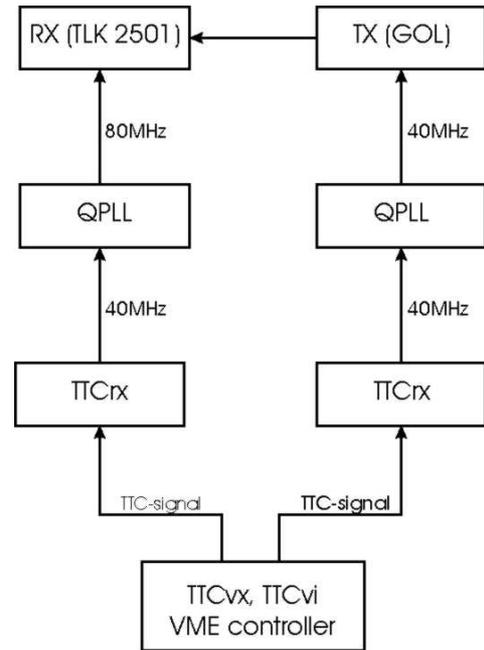
Figure 5 : BER test set-up
